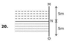
Two liquids of densities  $\rho_1$  and  $\rho_2(\rho_2=2\rho_1)$  are filled up behind a square wall of side 10 m as shown in figure. Each liquid has a height of 5m. The ratio of the forces due to these liquids exerted on upper part MN to that at the lower part NO is (Assume that the liquids are not mixing):
