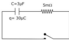
The circuit shown in the figure consists of a charged capacitor of capacity 3  $\mu F$  and a charge of 30  $\mu C$ . At time t = 0, when the key is closed, the value of current flowing through the  $5M\Omega$  resistor is 'x'  $\mu A$ .
