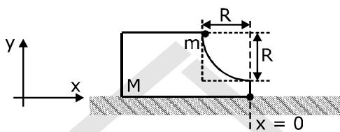
(A) The velocity of the point mass  $m$  is :  $v = \sqrt{\frac{2gR}{1 + \frac{m}{M}}}$
